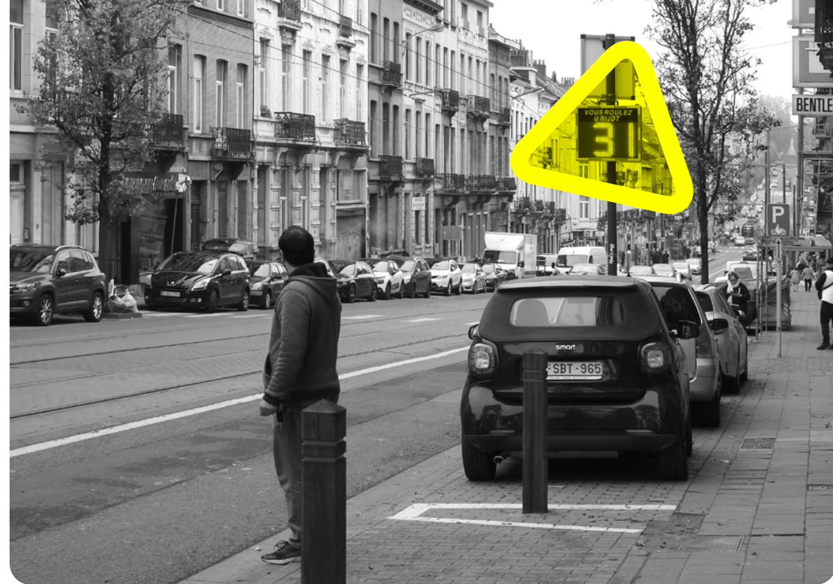
The speed control display blinks red indicating a car surpassing the 30 km speed limit – Iván Tosics
