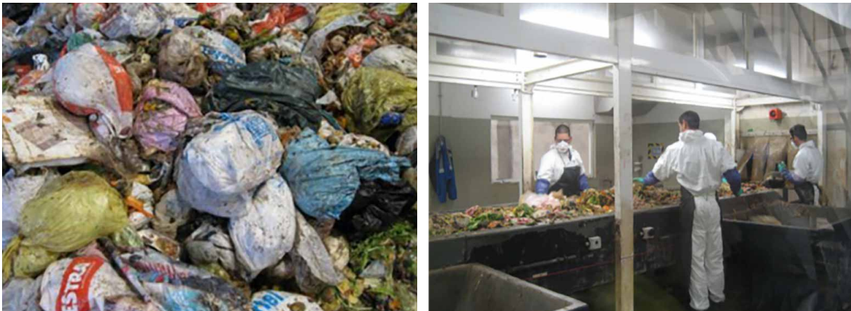
Figure 6: Valorsul AD plant in Lisbon, Portugal. Left – incoming waste. Right - manual sorting cabin (VALORGAS 2012b)
