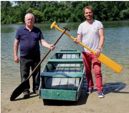
A traditional fishing dinghy, locally known as a 'ladik' can be made from riverine plastics. Unlike its wooden counterparts, this plastic boat requires little to no maintenance.
